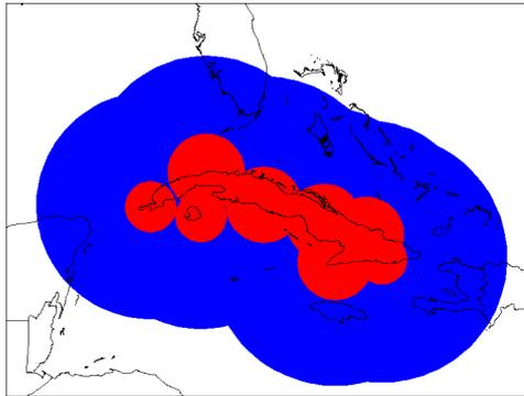
Fig. 1 Surveillance (blue), and Quantitative (red), coverage of Cuban Radar Network.
