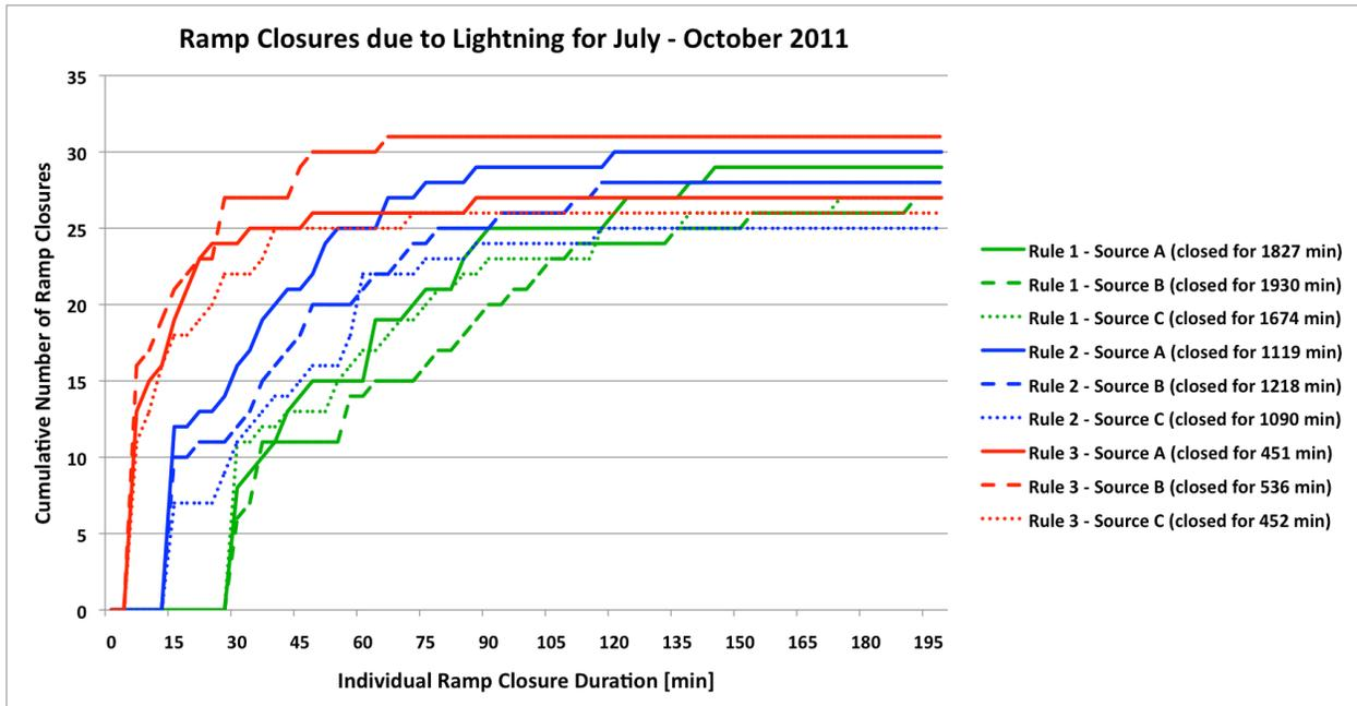
**Figure 2.** Ramp closures due to lightning threat near Airport X. Shown are the cumulative ramp closure distributions based on three different operator safety rules and three sources of lightning information. The total ramp closure duration for each combination is listed in parenthesis as well.
