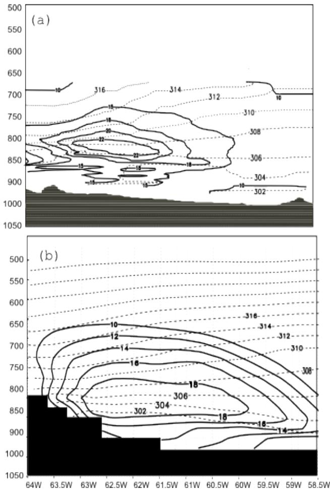
FIGURE 1 - Cross section of Zonal wind ( normal to the figure plane ) in m/s and isentropic lines (K) on 02 Feb 2003 at 12Z. a) Interpolate from NOAA P-3 aircraft data; ) Simulated by WRF mode.
