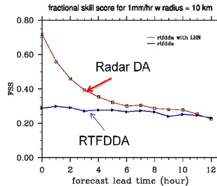
Fig. 1 Fractions Skill Score (FSS) for hourly-accumulated precipitation with the threshold of 1mm and a radius of influence of 10 km. Two runs over a period of 12 days during June 2010 in the Rocky Mountain Front Range region are compared for the standard RTFDDA without radar data and the upgraded version with radar reflectivity data assimilation through latent heat nudging (Courtesy of Mei Xu).
